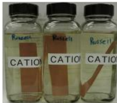
Figure 4. Color throw was observed after the HCl soaking for the cation membrane
