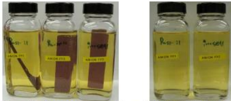
Figure 5. Color throw of the Anion membrane were observed after NaCl and NaNO 3 soaking.
